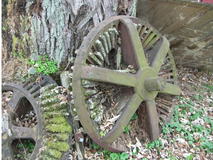
Figure ____ Discarded pair of hybrid nineteenth century bevel gears from the Dillar-Heishman Mill near Carlisle, Cumberland County, PA owned by Bill Foshag. This mill was originally built about 1800 but likely had an earlier 18 th century structure on the site. These bevel gears were part of the mill's turbine water drive which had replaced an earlier conventional wooden water wheel. (Photographed by the author and used with permission from the owner).
