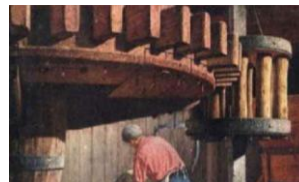
Large spur gear driving a lantern pinion gear
