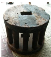
Lantern gear From Livezey's Mill
