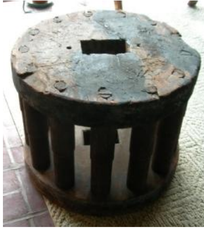
Figure ____ The only surviving component from Livezey's Mill, a lantern gear that was being used as a lamp table in Mike Firth's home. The rectangular central hole accepted a shaft with those dimensions so the gear would securely turn the shaft. This gear was about 18" high and nearly 2' across. The rounds show a step-notch indicating wear caused by the cogs driving them on the larger cog wheel. (Photographed by the author).
